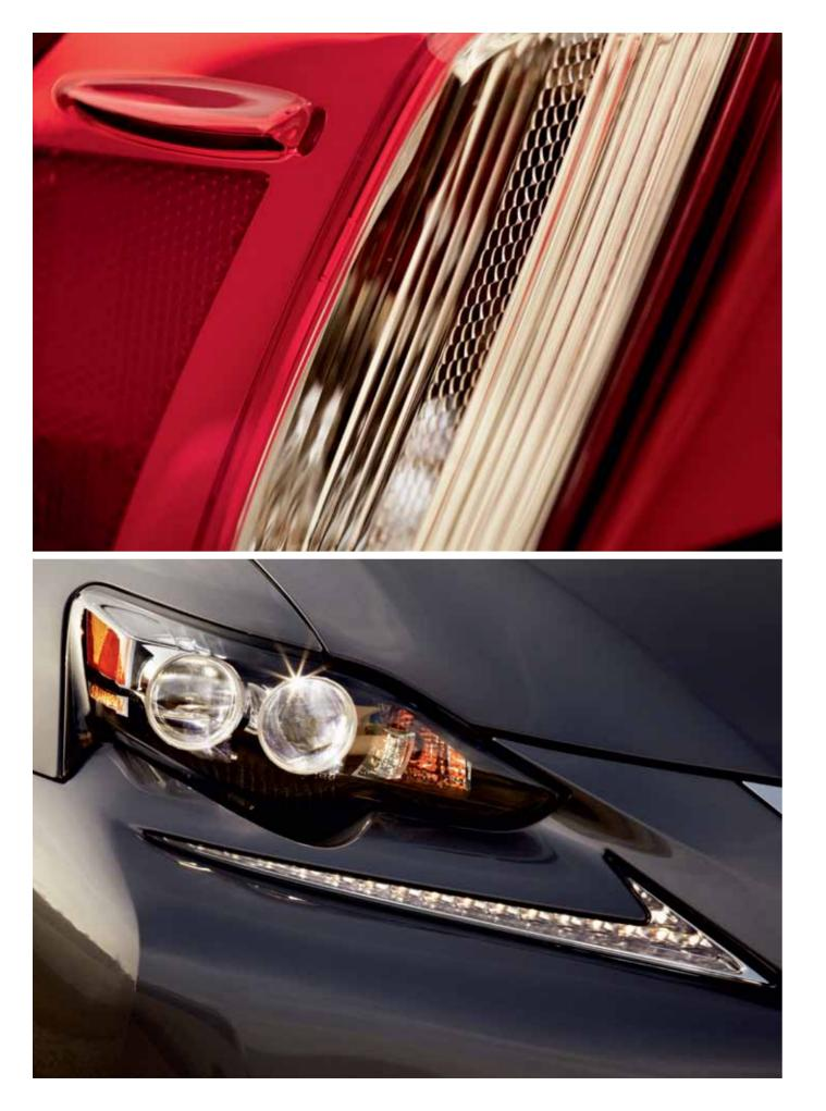
DAYTIME RUNNING LIGHTS The L-shaped daytime running lights (DRL) on the frontal treatment were designed to be shaped like an arrow, helping form a bold and speedy visual expression. Unlike the format on its predecessor, the lights on this IS are housed independently from the headlights.
