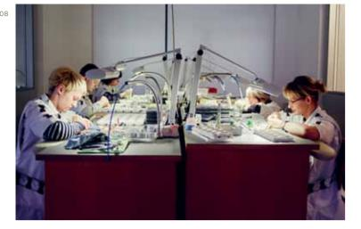
08 NOMOS watchmakers, in branded white overalls, work with minute components to create timepieces 09 A finished watch is cleaned and inspected 10 Tiny timepiece components sit in a glass jar; NOMOS is one of only a handful of local watch manufacturers that create their own parts
