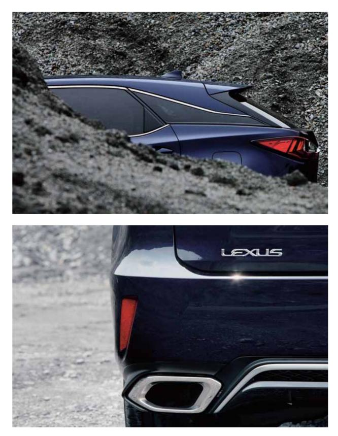
Meticulously crafted, the jewel-like taillights of the high-grade RX highlight a totally restyled end. The LED turn signal lights are sequential: meaning they illuminate in order from the inside to the outside, conveying the change in direction of travel.
